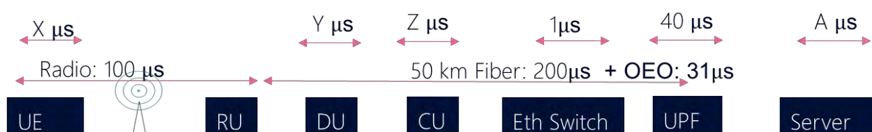
Figure 7-2: Latency components of a distributed RAN
