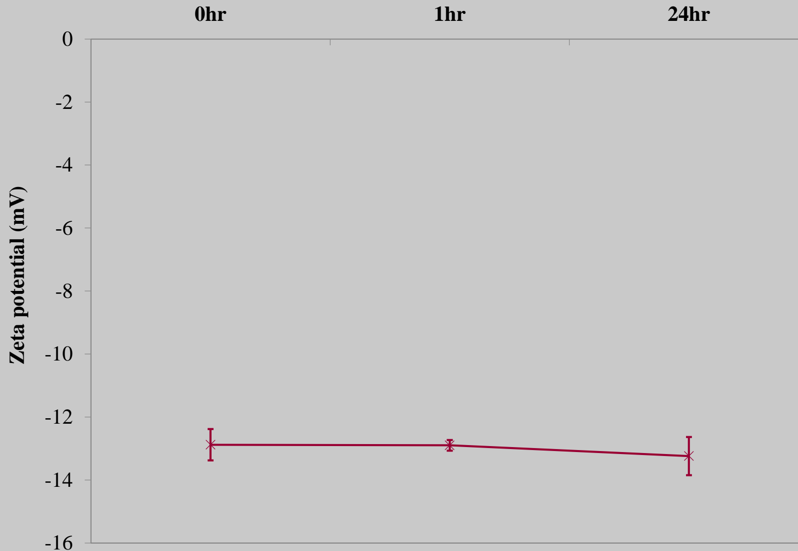
Fig 10: Zeta potential measurements of Alhydrogel in R10 medium following 0, 1 & 24hrs incubation (37°C). Error bars represent the \pm SD where n = 5 .
