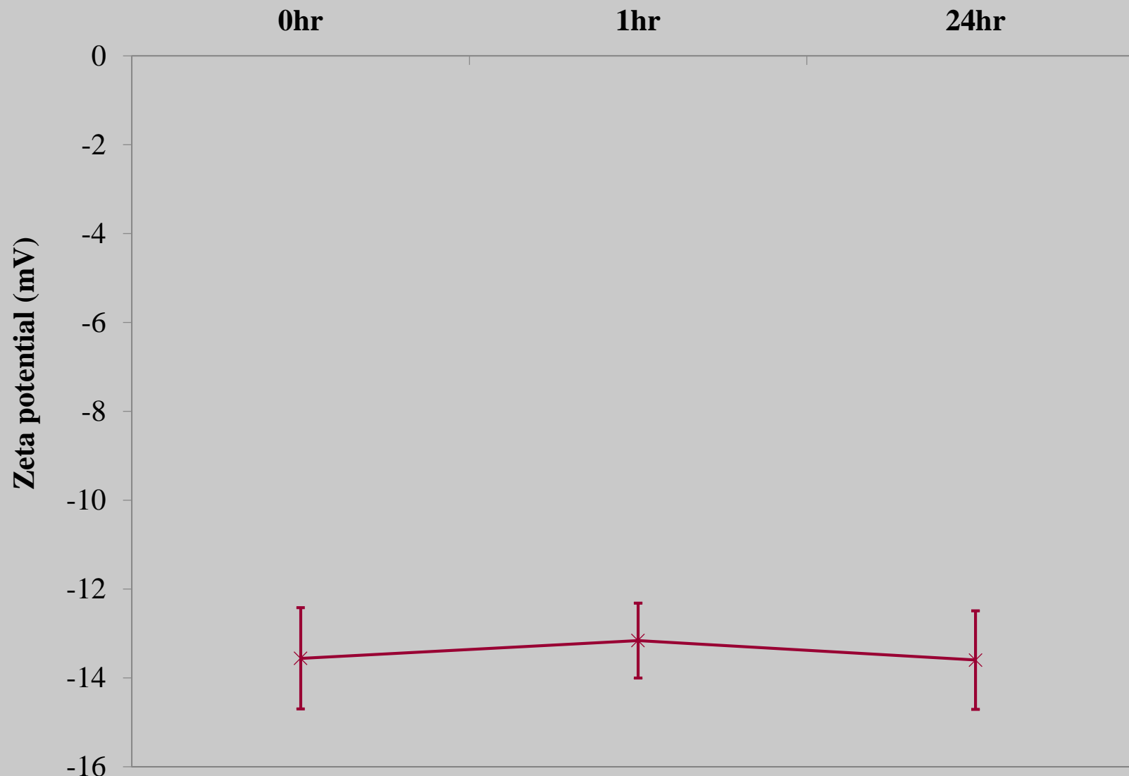
Fig 14: Zeta potential measurements of Adju-Phos in R10 medium following 0, 1 & 24hrs incubation (37°C). Error bars represent the \pm SD where n = 5 .
